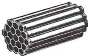
Figure 5 - Diagram of Round Tube Honeycomb Radiator.
