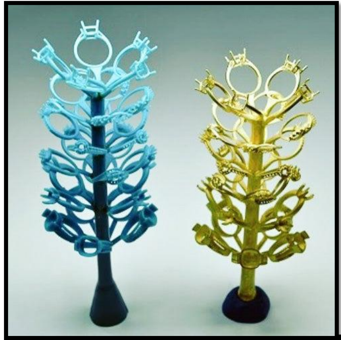
Figure 5 Wax casting tree (Hathaway, 2024)
