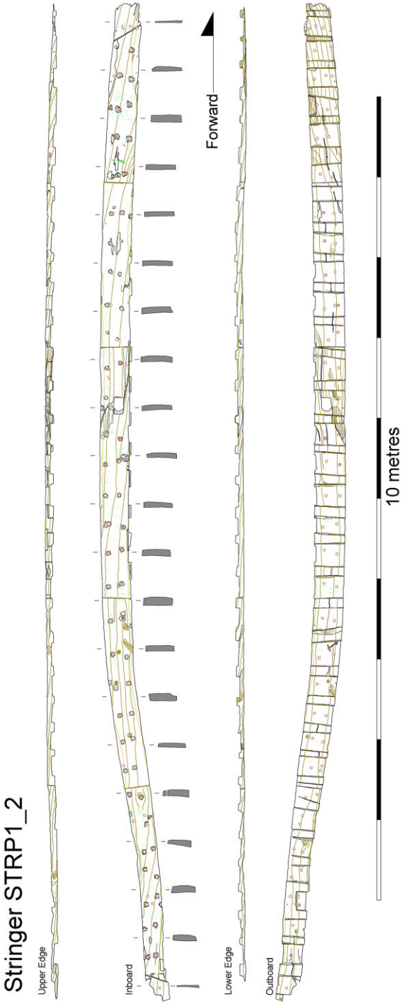
Figure 25. Stringer STRP1_2, with rebates for the mast-step braces visible along the lower edge. (Toby Jones)
