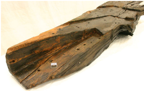
Figure 13. Starboard side of the stem showing scarf to keel and rebates for hull planks. (Stuart Churchley, Newport Museums and Heritage Service)
