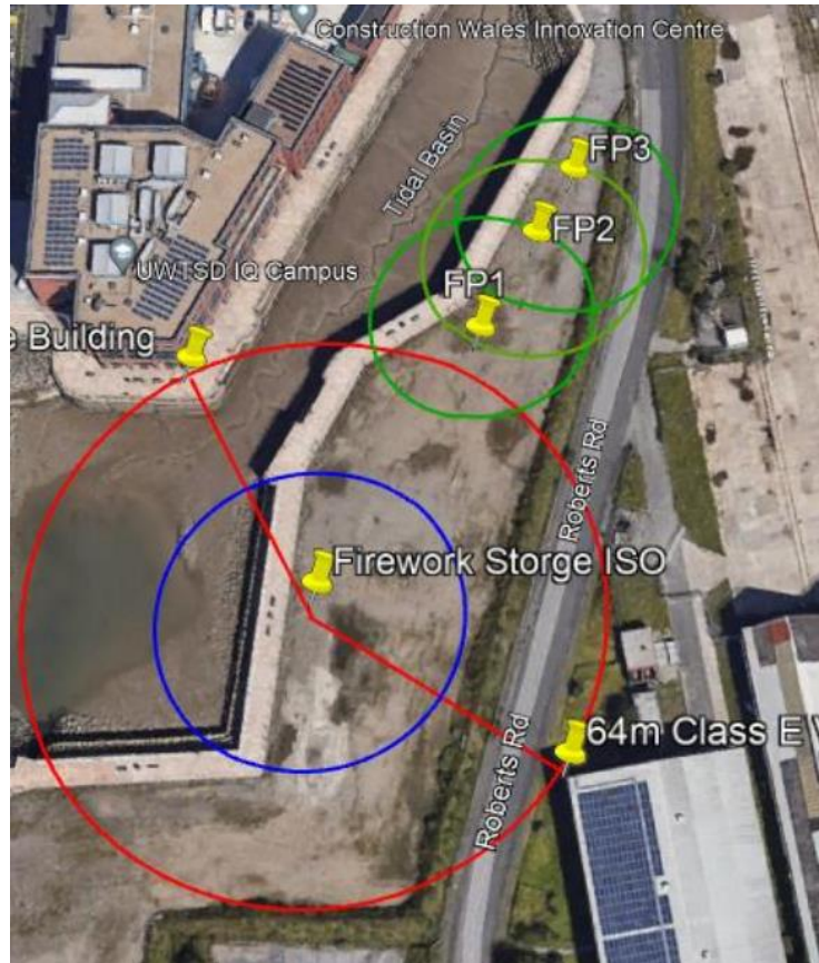
Figure 11: Detailed satellite view showing interaction of storage area with other areas.
