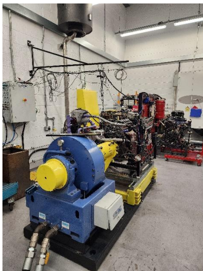
Figure 1 photo of the W230 Eddy current dynamometer (photo taken by Student)
