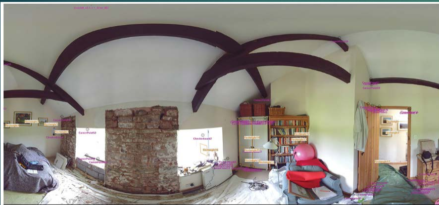
Laser scan output images which measures the total interior space to within 2mm and creates linked continuous images
