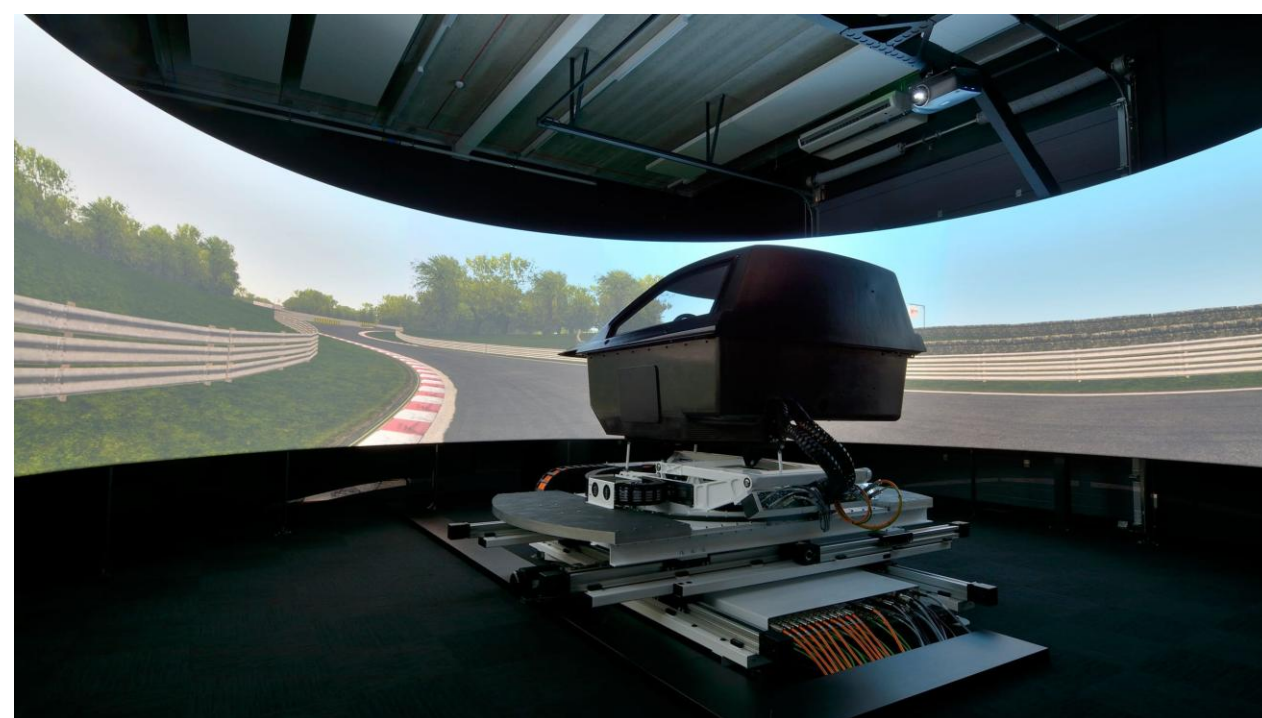
Figure 3 –Driving Simulator is a form of testing that different manufactures test their vehicle before putting the vehicle out to the real world. This way the manufactures can discover any fault of the vehicles handling prospect.
