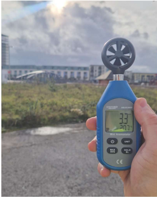
Figure 20: Measuring wind speed using an anemometer (Photo credit: D. Dennehy)
