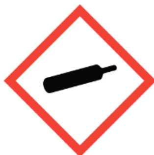
GHS04 Compressed Gas
