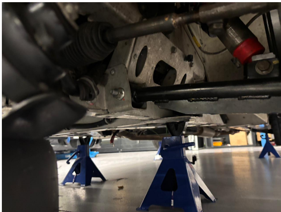
Figure 5: Underside view of the Morgan CX-Generation aluminium chassis on axle stands. The flat bonded-and-riveted aluminium panels are clearly visible, along with the suspension lower arm, coilover spring (red), and chassis bracket with lightening holes.
