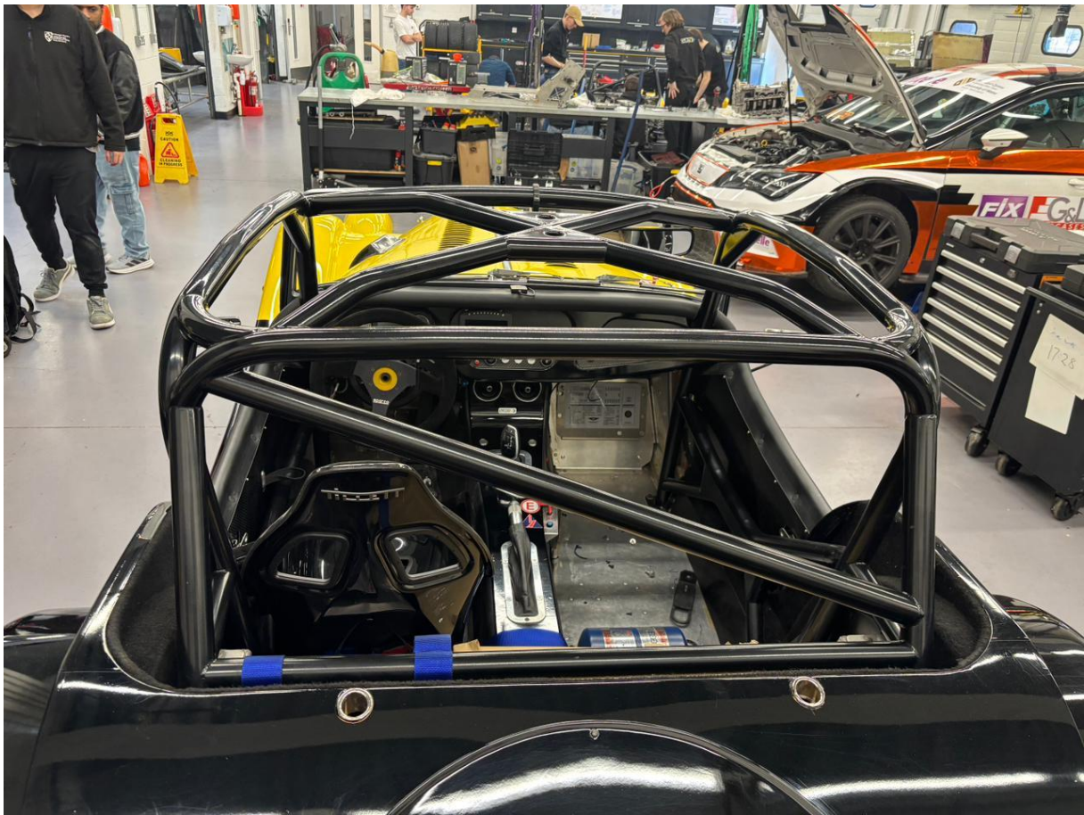
Figure 2: Rear view of the full multi-tube steel roll cage installed in the UWTSD Morgan. The main hoop, diagonal cross-braces, and side members are visible. The Tillett racing seat, Sparco steering wheel, and exposed aluminium CX-Generation chassis floor can also be seen within the cockpit.
