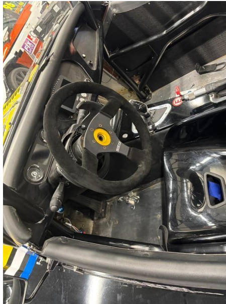
Figure 3: Cockpit interior showing the Sparco suede racing steering wheel (no airbag), Tillett carbon composite racing bucket seat (driver side only — passenger seat removed), roll cage side member, carbon fibre cockpit side panel, and the bare aluminium CX-Generation chassis floor. The Lifeline fire extinguisher pull cable is visible at lower left, and the Motorsport UK kill switch sticker is on the right side panel
