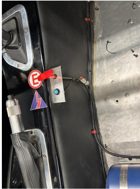
Figure 8: External fire extinguisher pull handle (red T-bar, centre) and external kill switch (red push-button, below it) mounted on the top of the scuttle/body between the windscreen and bonnet. The Motorsport UK fire(E) symbol sticker and electrical hazard triangle sticker are also visible, as required by Motorsport UK General Regulations.
