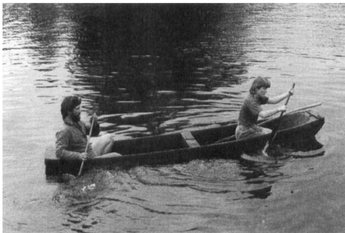
Figure 2. The Clapton dugout boat replica undergoing familiarization trials on the River Thames using replica oak paddles.
