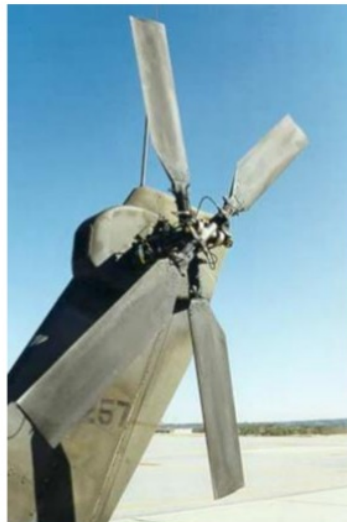
Figure 4 - Apache tail rotor arrangement
