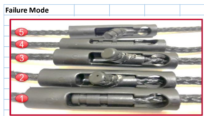
Figure 24 Images Supplier took of failure modes of samples that have undergone the locking mechanism test
