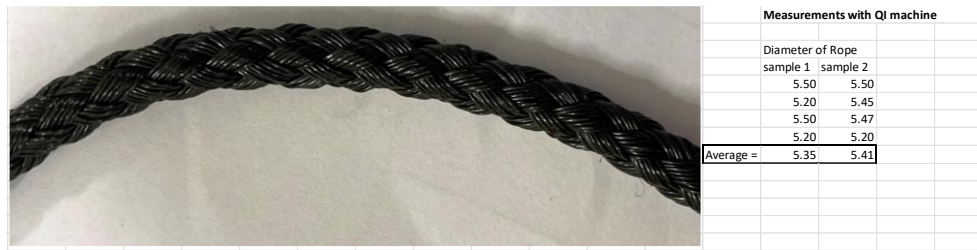
Figure 39 Measurements of Rope Diameter (old rope)
