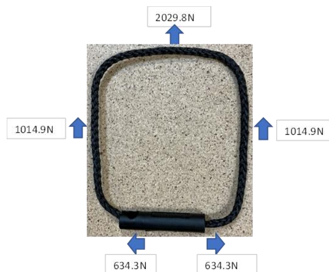
Figure 18 Force Calculations for Continuous Load Test Following EnerSys' requirement
