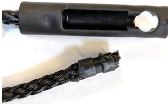
Figure 34 Sample 1 - Failure Mode 1 - Newport Physical Testing
