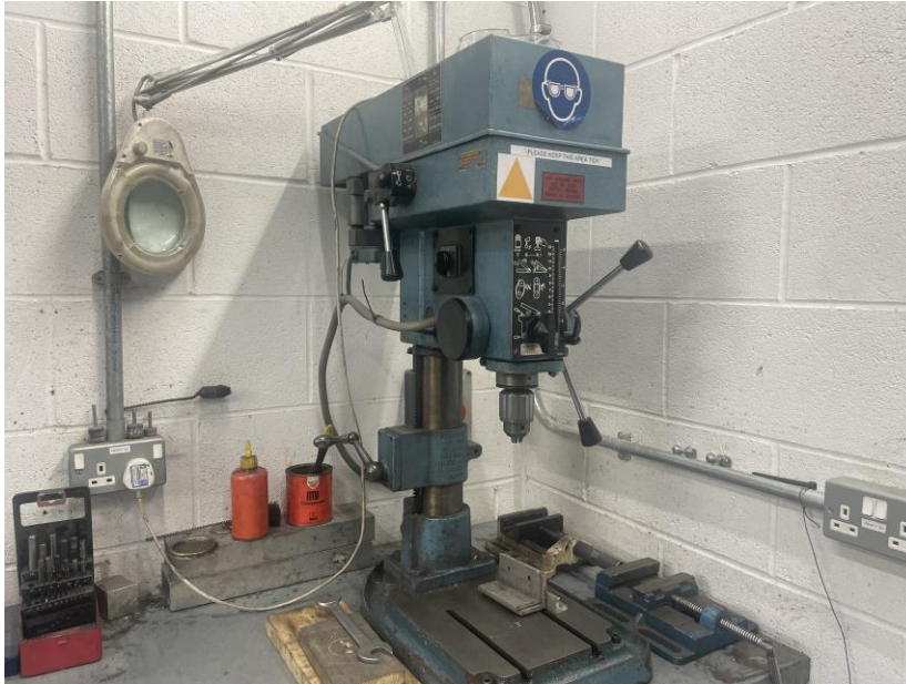
Figure 3-1 Pillar Drill in Fabrication Workshop (Flye, 2024)
