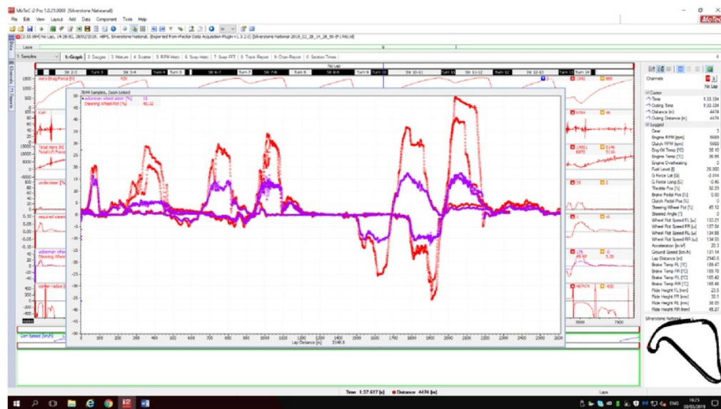
Appendix 7c - A graph showing the correlation between Ackerman steering percentage, wheel steer percentage and lap distance for setup F1,R6
