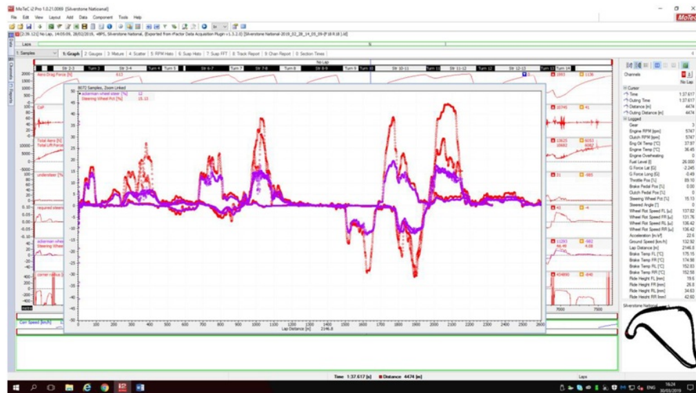
Appendix 7a - A graph showing the correlation between Ackerman steering percentage, wheel steer percentage and lap distance for setup F18, R18
