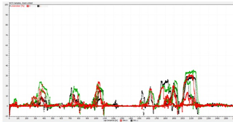
Figure 19 - A graph showing the correlation between understeer and lap distance for three setups
