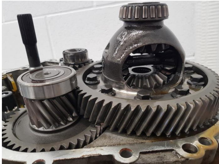
Figure 61 Reverse gear connection to the differential drive gear.
