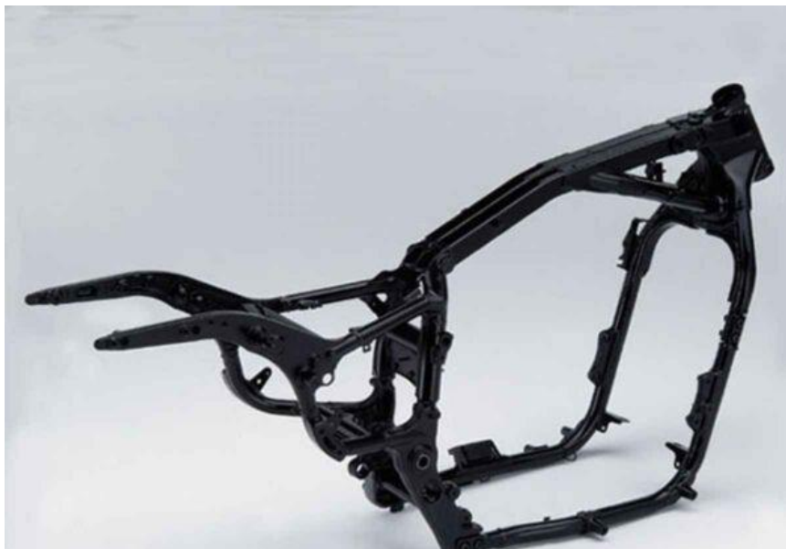
Figure 2-2 This shows the double down pipes and frame itself.
