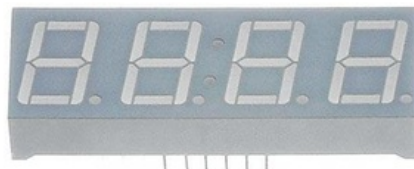
Figure 16: Example of 4 digit 7 segment display [16]
