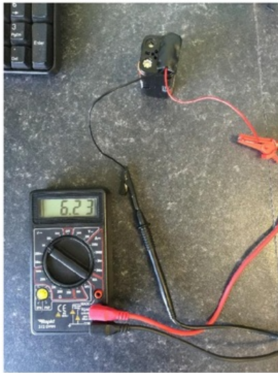
Figure 43: Battery supply voltage
