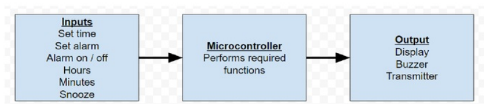
Figure 4: Digital alarm clock block diagram
