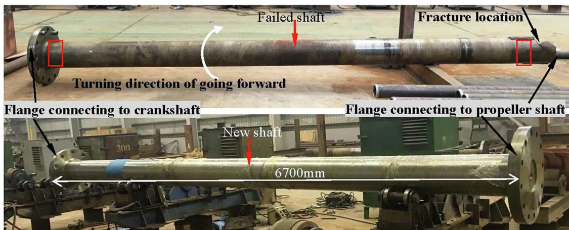
Figure 4-1 - Failed Bulk Carrier Shaft Highlighting Fracture Location, Compared to New Shaft [4]
