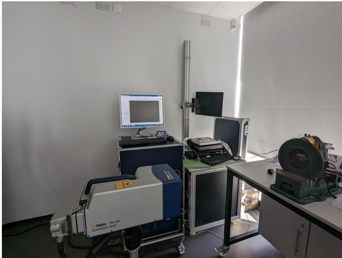
Figure 1 : Laser Doppler Vibrometer Equipment
