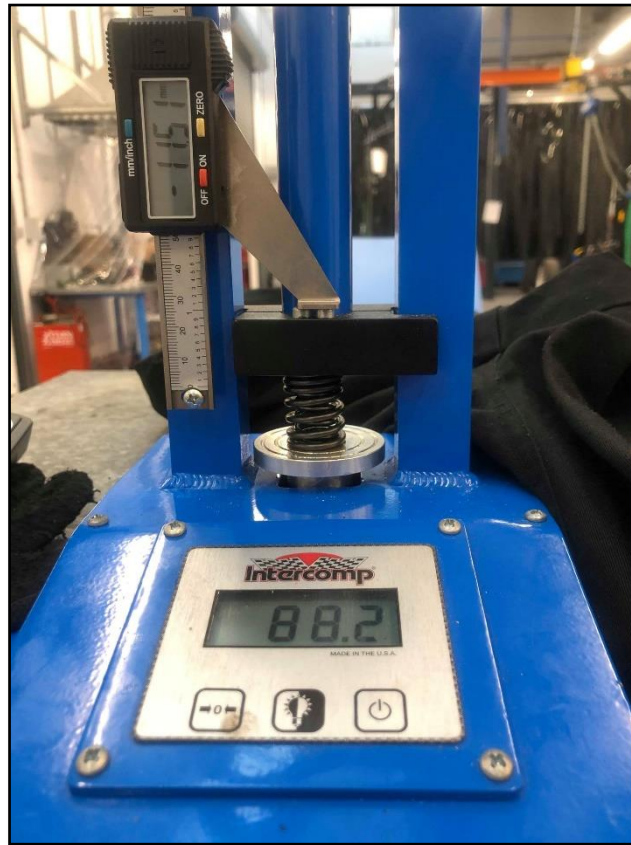
Figure 49 Measuring Intake Valve Spring Rate
