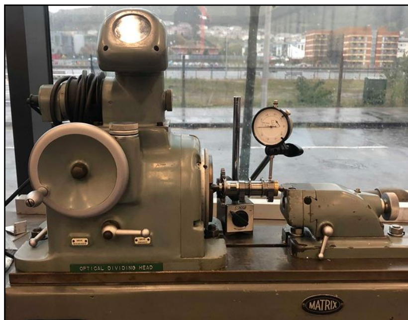
Figure 45 Measuring Intake Cam Profile
