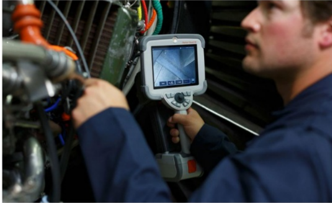
Figure 14. Technician performing visual NDT on an aircraft engine (McMenamin, 2015)
