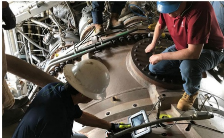
Figure 13. HD Video borescopes of a gas turbine (Fitzgerald, 2018)
