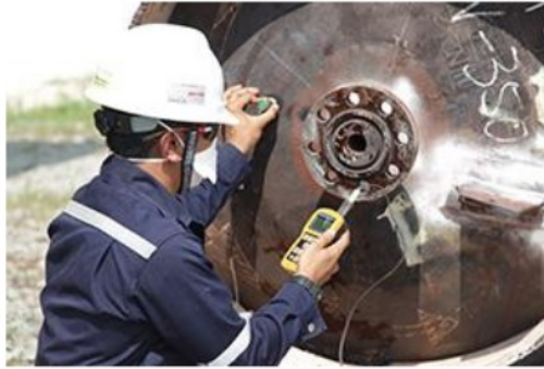
Figure 10. Ultrasonic testing of a components thickness (NUSATEK, 2019)
