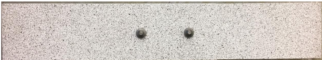
Figure 31 – double riveted coupon
