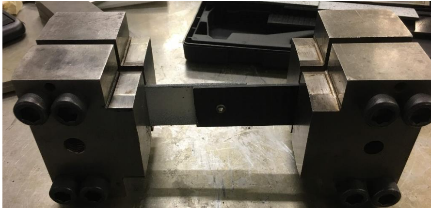
Figure 38 – Grips holding coupon in place.
