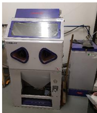
Figure 22 – Shot blasting machine on left, vapour blasting machine on right.
