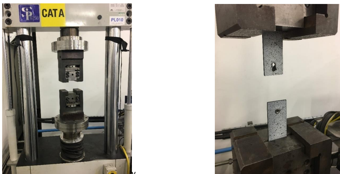
Figure 15 – Constant load-rate machine with grips on left, tensile tested coupon on right.
