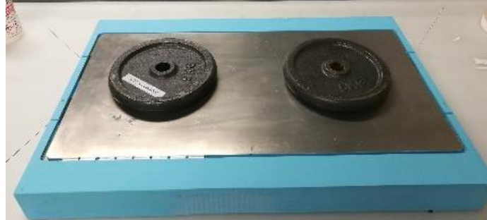
Figure 34 – Metallic plate and weights on coupon
