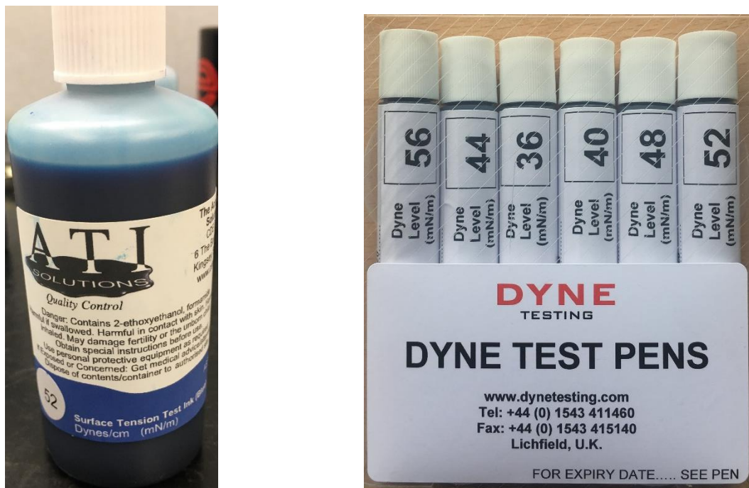
Figure 27 – Dyne pen liquid on the left, dyne pens on the right.
