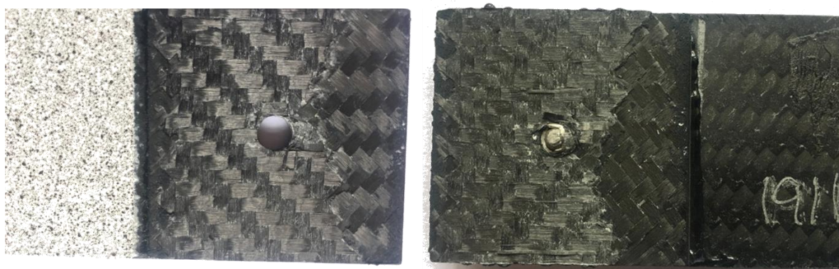
Figure 42 – First Ply failure, part 191128_14
