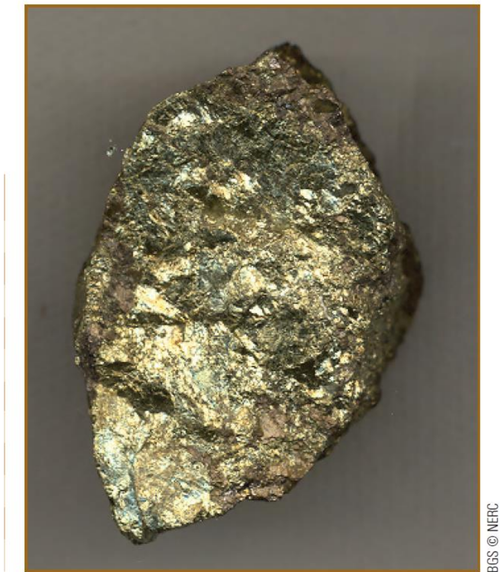
Figure 2 Chalcopyrite, the primary ore of copper.
