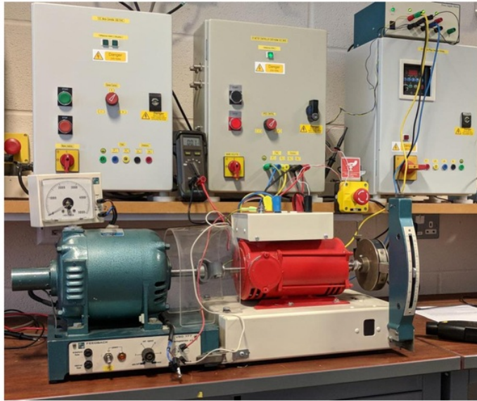
Figure 6 - Test Motor and Drive
