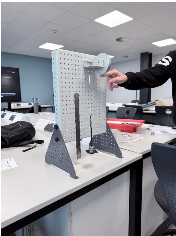
Seen above, is image 2, which shows the assembly at its bottom-most point, just before the residual energy in the flywheel brings it back up to h_2 .
