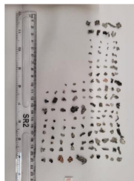
Figure 3: Fragments produced by the munition
