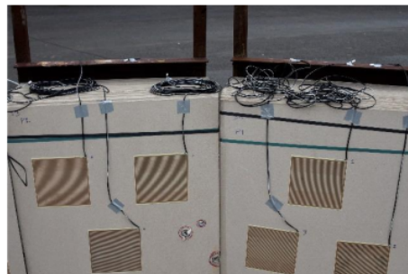
Figure 2: Velocity foils attached to witness packs at COTEC
