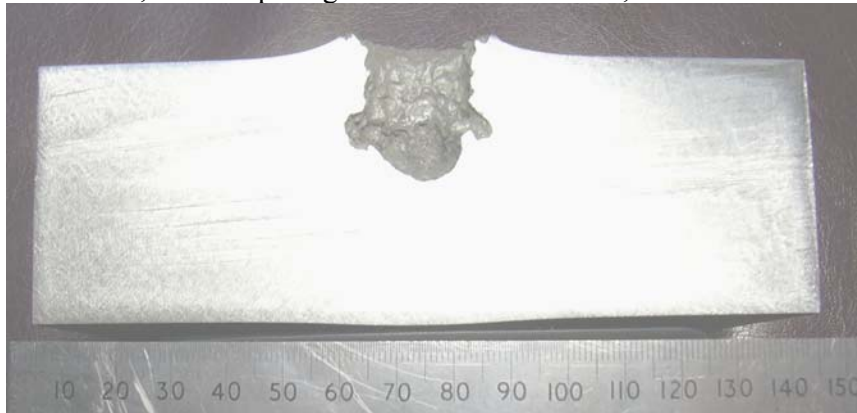
Figure 1. Sectioned aluminum target from Test VIII. Standoff 1.5 C.D.
