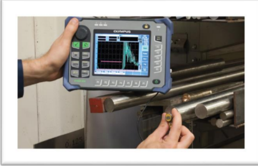
Figure 4. – Typical portable UT equipment being used to test extruded round bar for defects (Quality Mag, 2015).
