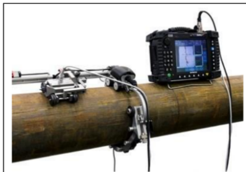
Figure 10. – Image of ECA being utilised to test pipework for defects while in operation with little to no preparation (Morgan Ward, 2019)
