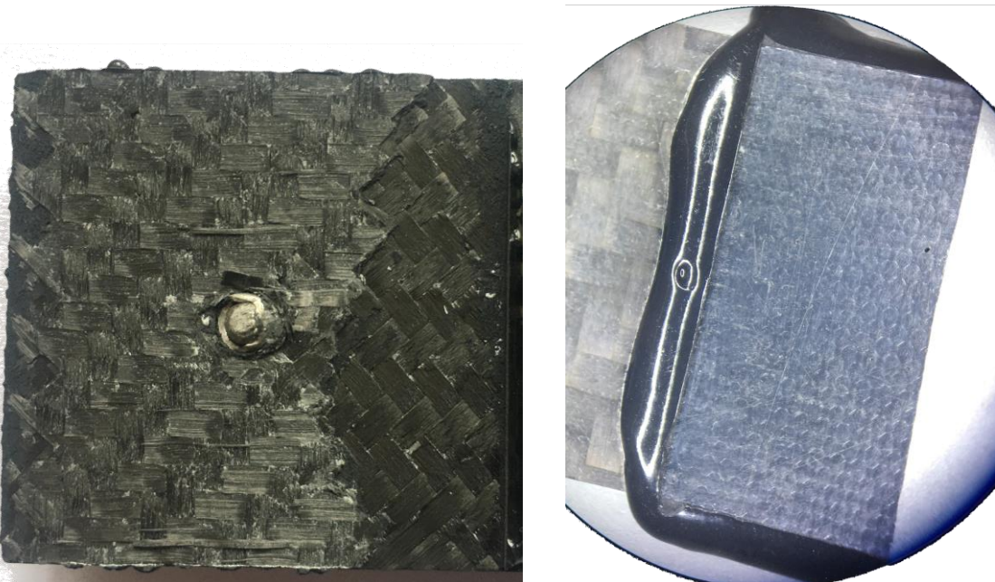
Top left shows a failure of the first ply of the coupon, top right is an adhesive failure between the glue and the carbon fibre, this kind of failure happens when the treatment of the material beforehand is not enough.
