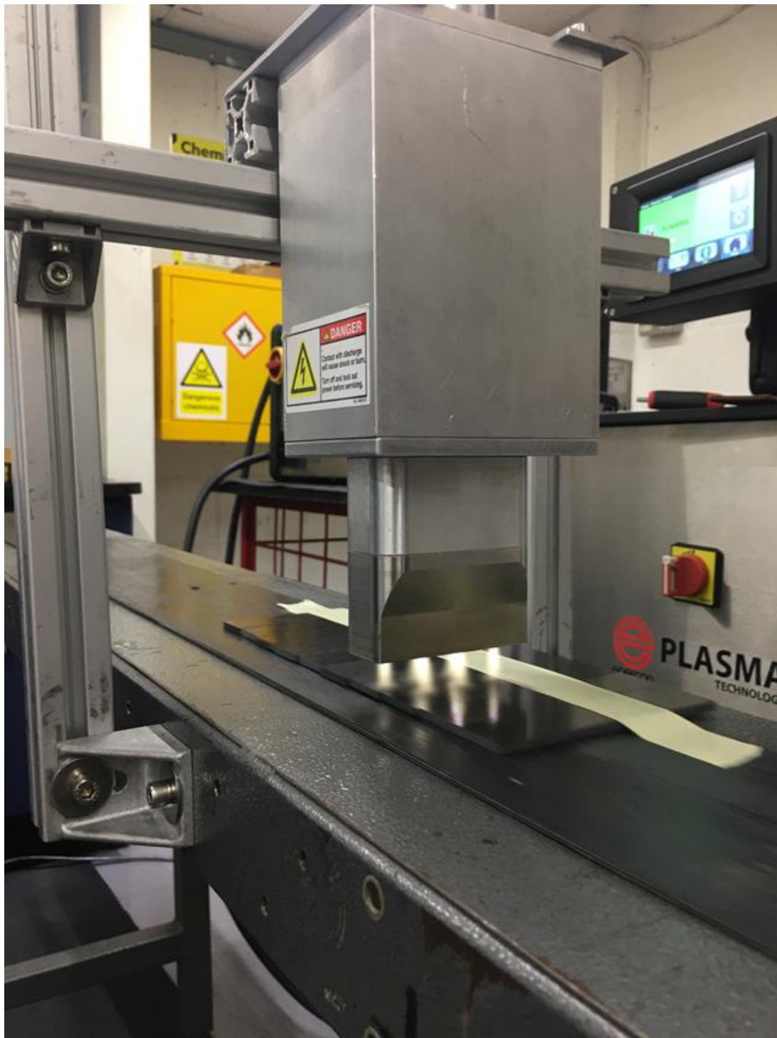
Plasma treatment of coupons, multiport blown ion plasma
