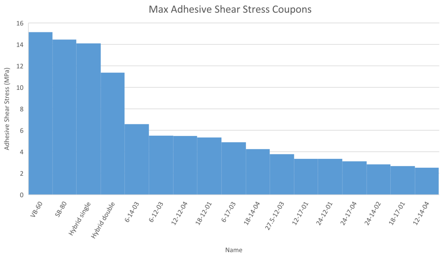
The above graph, compares the difference of adhesive shear stresses between all the different joining technologies, the best joining technology was bonded coupons with a vapour blasted treatment.
