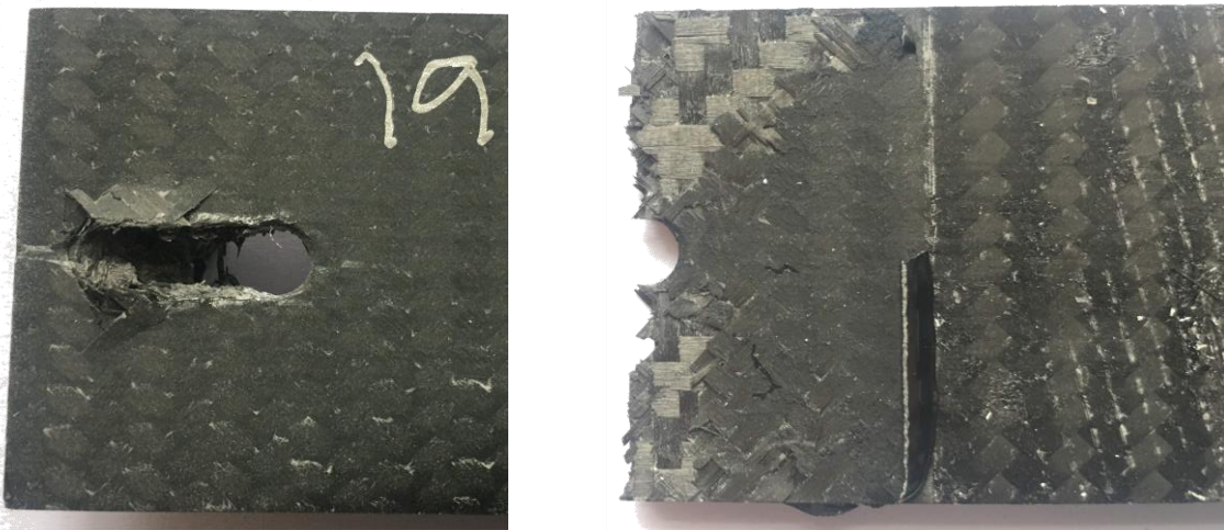
Top left shows a tear out of the material where the rivet was originally, top right is a structural failure of the coupon along the hole line.
