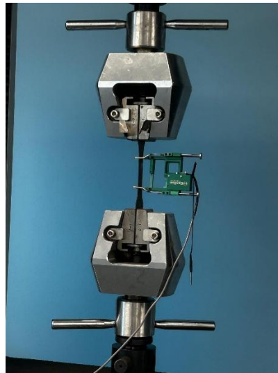
Figure 4.1: Denison tensile machine fitted with Epsilon clip-on extensometer (50 mm gauge length, 0.001 mm precision) for measurement during ISO 6892-1 tensile testing.
