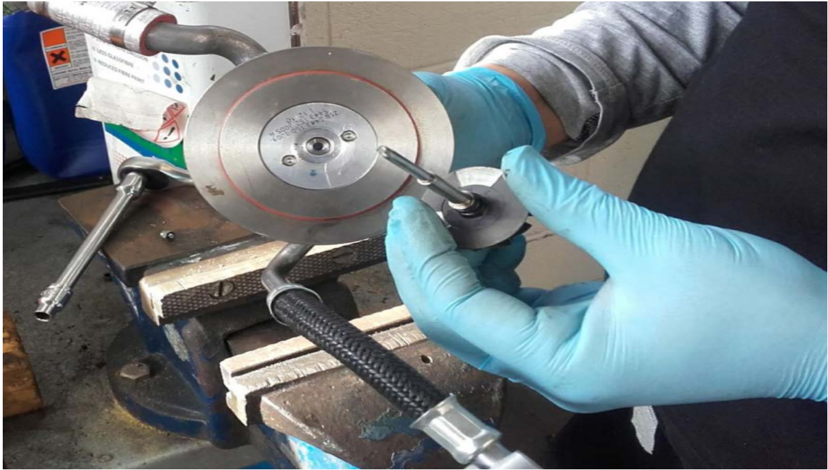
Figure (16) (Barsoum, 2018) the axis thread is French thread to prevent the axis lose both sides, keep them tight all the time.
