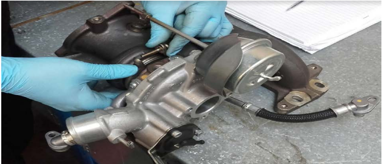
Figure (24) (Barsoum, 2018) after you fit the waste gate case fit the clamp metal to connect the body of the turbocharger.
