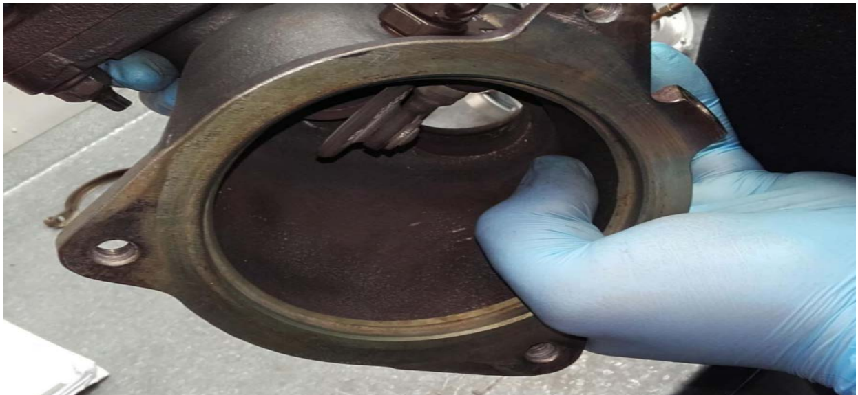
Figure (5) (Barsoum, 2018) here you can see waste gate, small emission gate to let the gas cycle go from turbine cavity move to another area.
