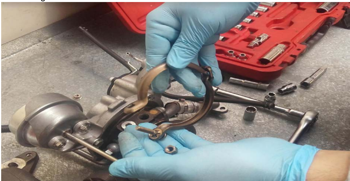
Figure (9) (Barsoum, 2018) Keep the metal clip totally jointed with nut, wisher and bolt.
