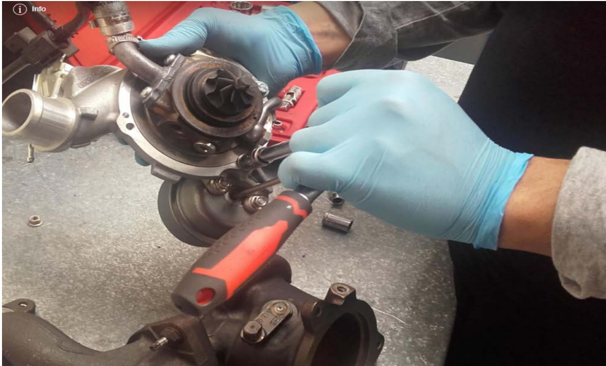
Figure (22) (Barsoum, 2018) always use the ratchet in the correct position which is 90 degrees for get good functioning.
