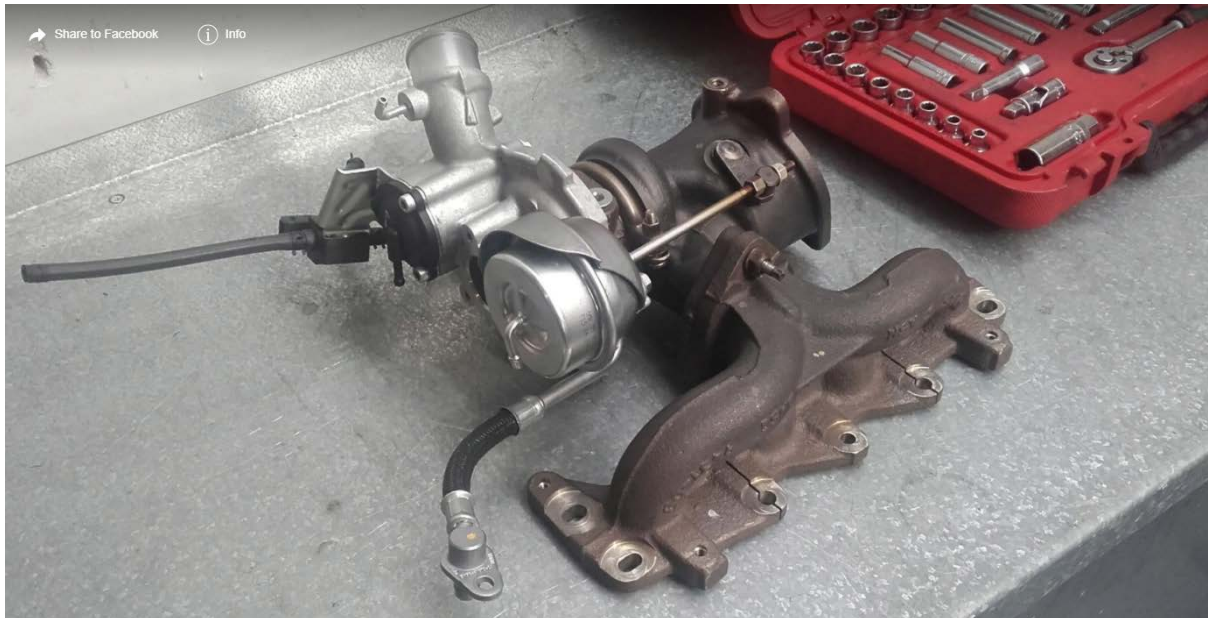
Figure (2) (Barsoum, 2018) the beginning start with the total turbocharger stripped from diesel engine.
