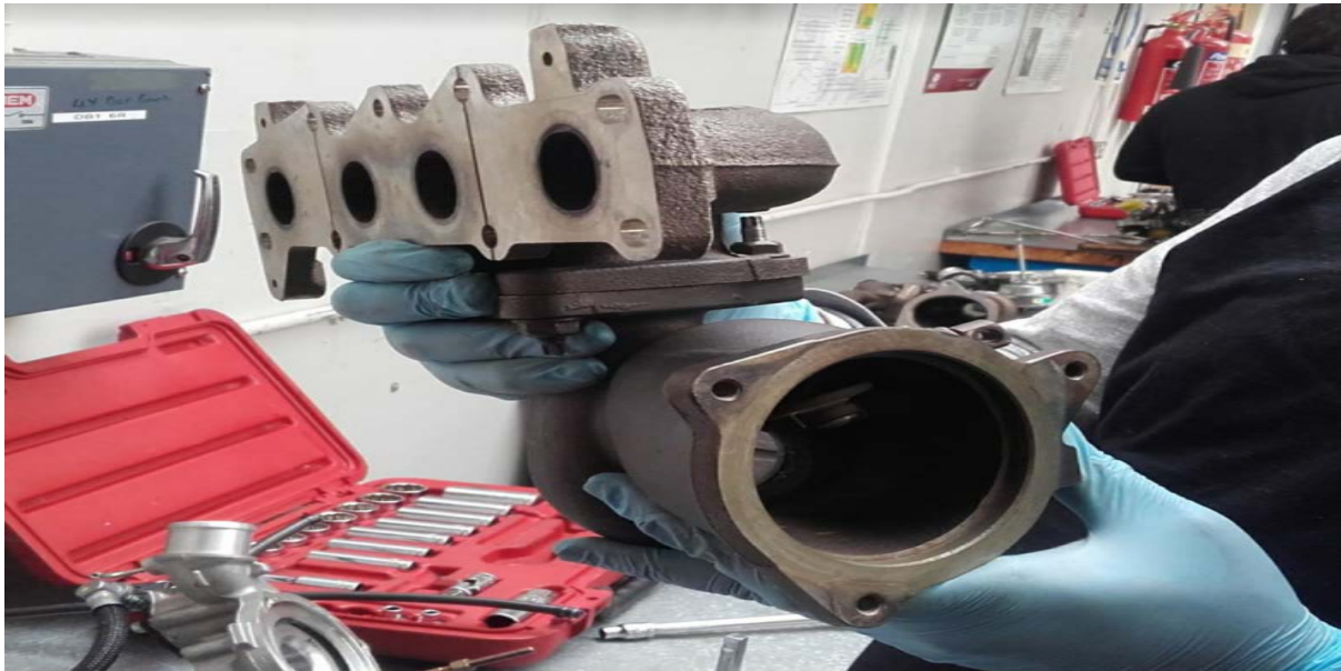
Figure (4) (Barsoum, 2018) the four cylinders emission outlet into manifold exhaust gasket connected to the turbocharger.
