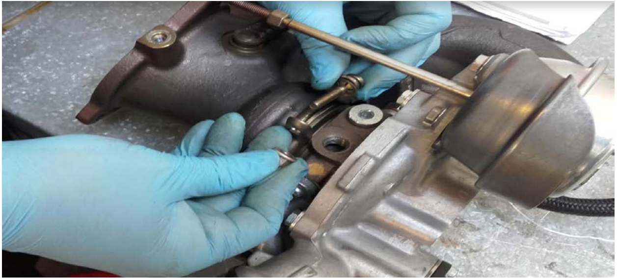
Figure (8) (Barsoum, 2018) move the bolt and wisher kindly and keep the bolt, nut, and wisher aside of the turbocharger.
