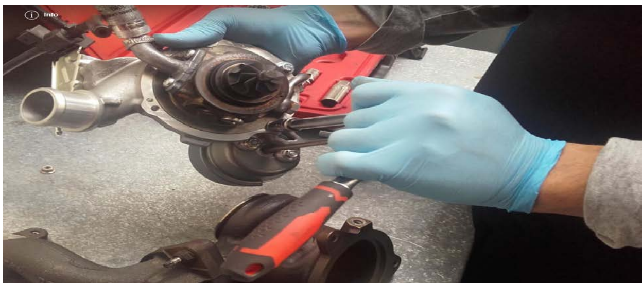
Figure (21) (Barsoum, 2018) tightly check all the bolt at the same torque to avoid any sort of air or exhaust gas leak while the turbocharger functioning.
