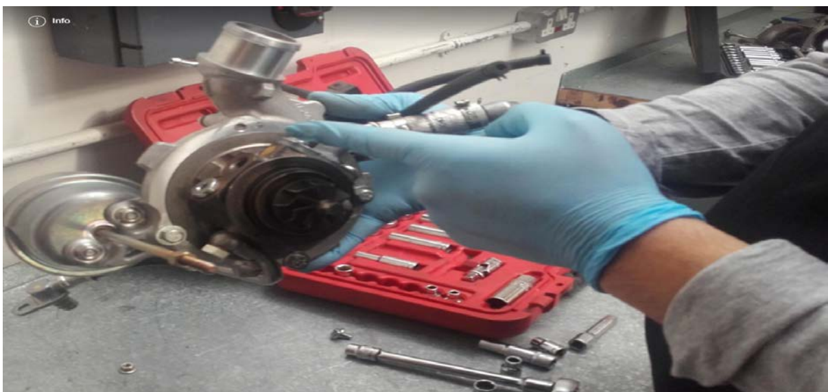
Figure (23) (Barsoum, 2018) check at the turbocharger case there no any sort of corrosion or rust and any cracks.
