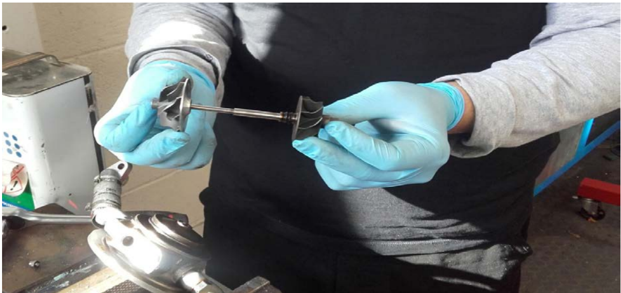
Figure (17) (Barsoum, 2018) compressor wheel ,spindle and turbine wheel ,the axis holding both sides of the flow circulation from the ambient inlet and exhaust turbine which guide increase the air flow into the engine when its rotation in the same axis.
