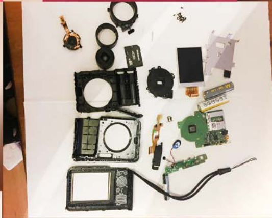
Lens, a shutter, an image sensor, CCD and CMOS imager, an LCD screen and a memory card
