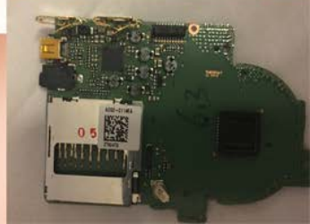
Glass fiber reinforced (fiberglass) epoxy resin with a copper foil bonded on to the one side
