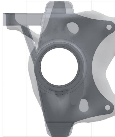
Figure 8-24 - Design 8 and final topology overlay
