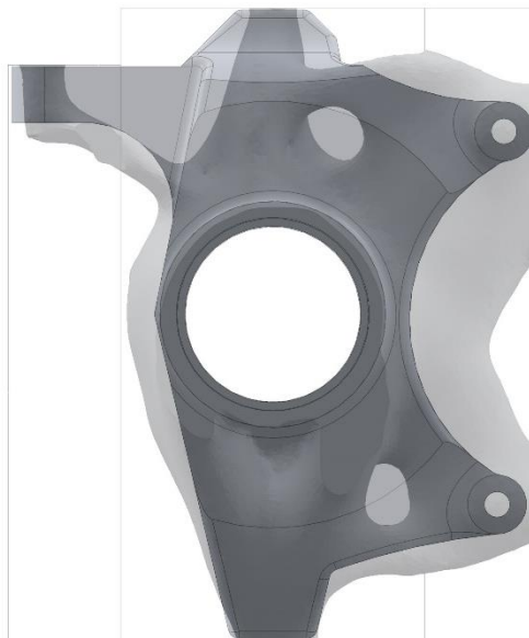
Figure 8-6 - Design 1 and final topology overlay
