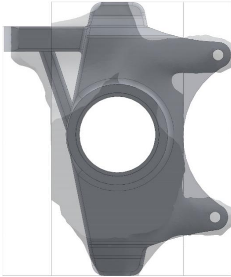
Figure 8-23 - Design 8 and second topology overlay
