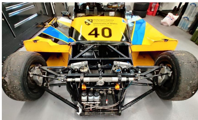
Plate 2-2 - MCR S2 front suspension geometry
