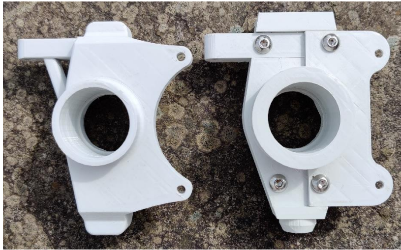
Plate 16-1 - 3D printed models of the original and new upright design (front)
