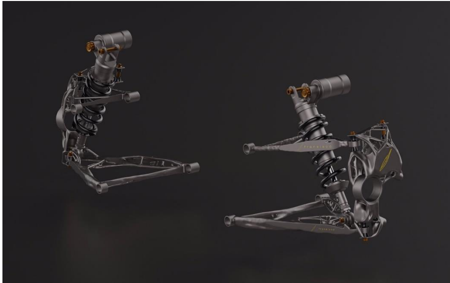
Figure 5-13 - Topologically optimized Lotus Elise S1 upright designed by Fransisco, manufactured by Carbon Performance (Peters, 2019)
