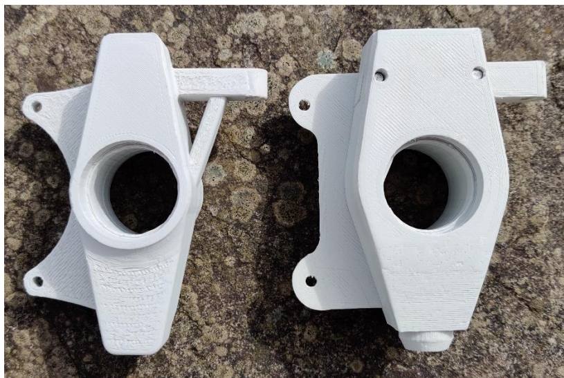
Plate 16-2 - 3D printed models of the original and new upright design (rear)
