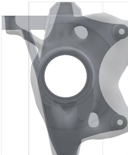
Figure 8-10 - Design 2 and final topology overlay
