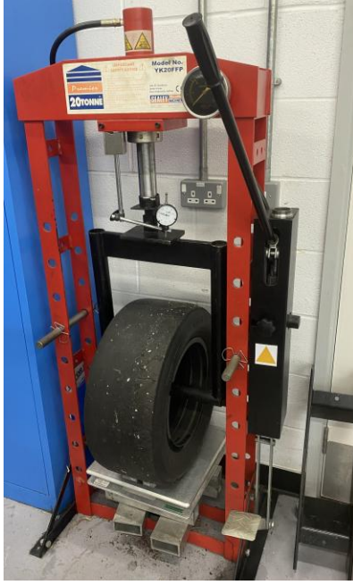
Figure 3.5: Left (a): Workshop measurement of tyre/wheel vertical stiffness and Right (b): steering-wheel-to-road-wheel angle calibration for the MCR #40.
