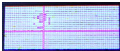
Figure 26: A scene containing the hot mug of water as observed by the Infrared Sensor. Dark pixels indicate a hotter, lighter indicate cooler.
