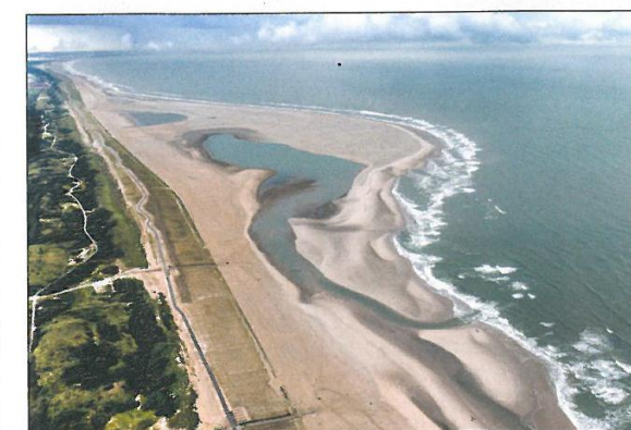
Figure 2. Delfland sand engine in October 2012 – sediment is being transported along the coast, young dunes are forming, pioneer plant species are beginning to settle and the lagoon is a nursery for flatfish ( https://beeldbank.rws.nl , Rijkswaterstaat / Joop van Houdt)
