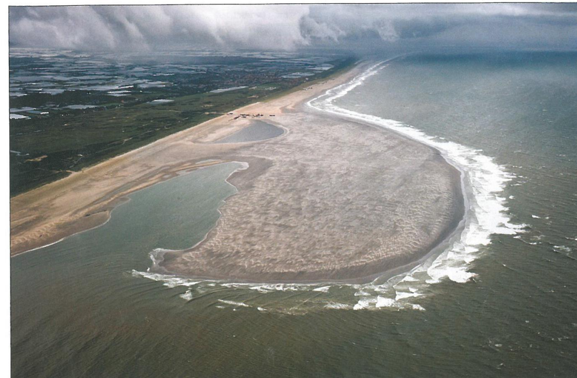
Figure 1. Delfland sand engine in July 2011, just after completion – a total of 20 million m 3 of sand was placed in front of the existing shore ( https://beeldbank.rws.nl , Rijkswaterstaat / Joop van Houdt)
