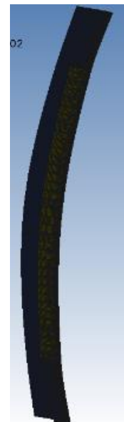
First order bending seen at 49.7Hz
