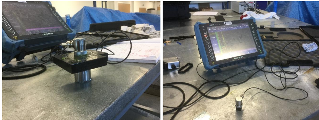
Figure 4-23: Measuring of the Speed of Sound. Through Transmission (L) & Backwall Reflection (R).
