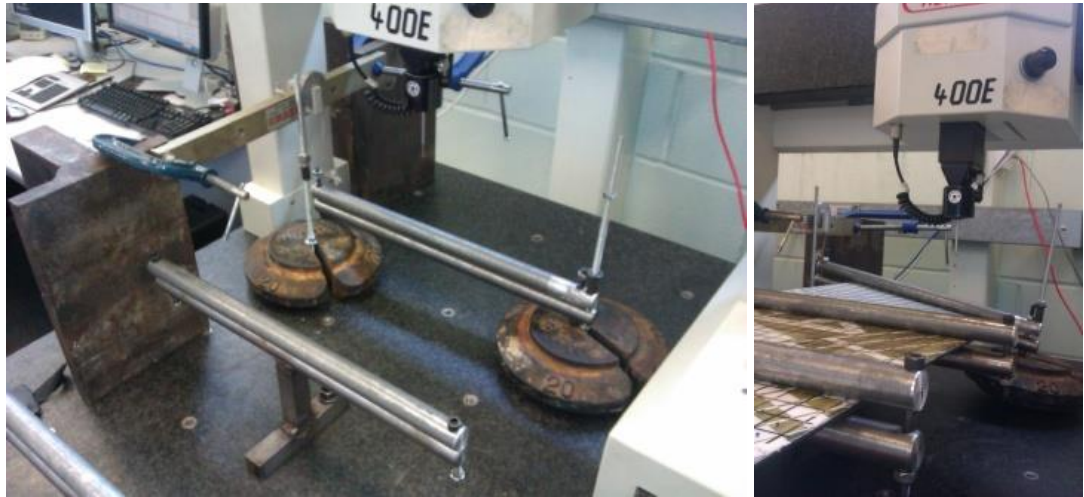
Figure 5-13: Measuring the Torsional Stiffness of the Boards.
