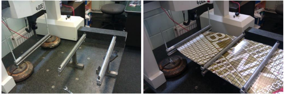
Figure 5-6: Measuring the Bending Stiffness (Regions 1 & 4).
