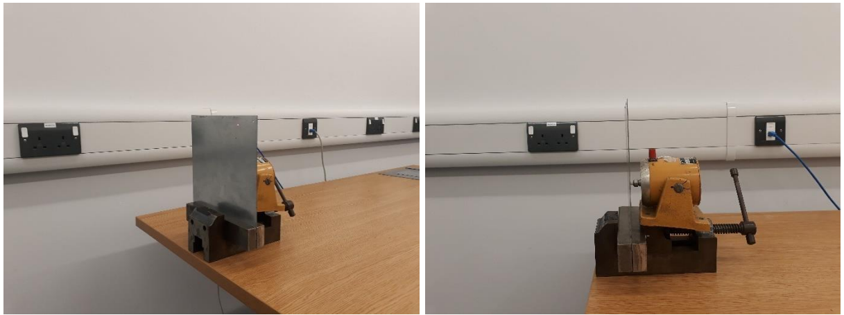
Figure 4-6: Vibration Testing Clamping the Plate Along One Edge.
