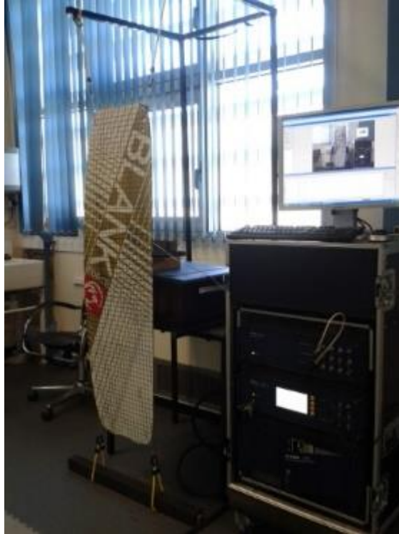
Figure 5-19: Vibrational Testing Set-up of the Boards.
