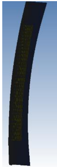
First order bending at 46.0Hz
