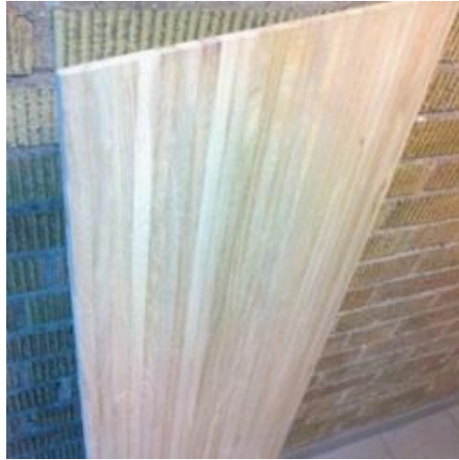
Figure 6-1: Paulownia Wood Core (123).
