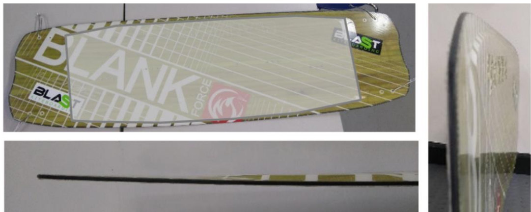
Figure 5-16: The Increased Depth in Regions 2 & 3 of the Glass Board.
