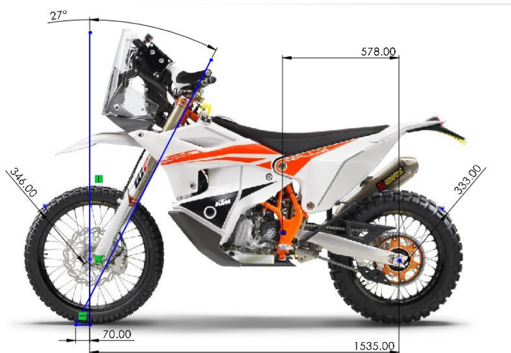
Figure 27: KTM 450 Rally geometry (image courtesy of www.amsmoto.co.uk ).
