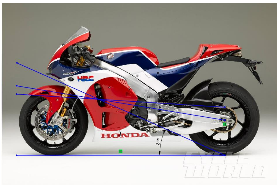
Figure 26: RC213V-S anti-squat angle (image courtesy of www.cycleworld.com ).
