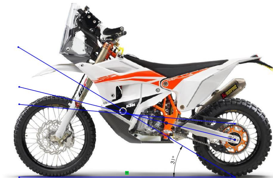
Figure 28: KTM 450 Rally anti-squat angle (image courtesy of www.amsmoto.co.uk ).
