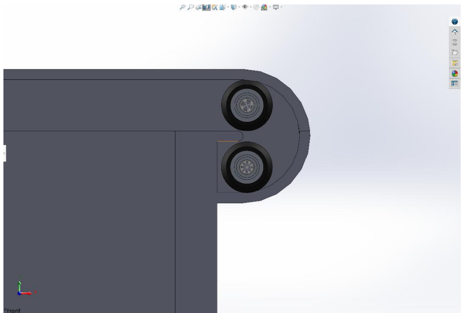
Figure 11 shows a close up of how the rollers make it round the arc to allow the lid to sit vertically down the side.
