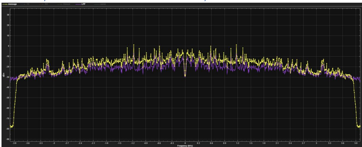
Figure 12: Spectrum Analyser view of the message and filtered signals in a DSB-SC simulation with noise present in the channel
