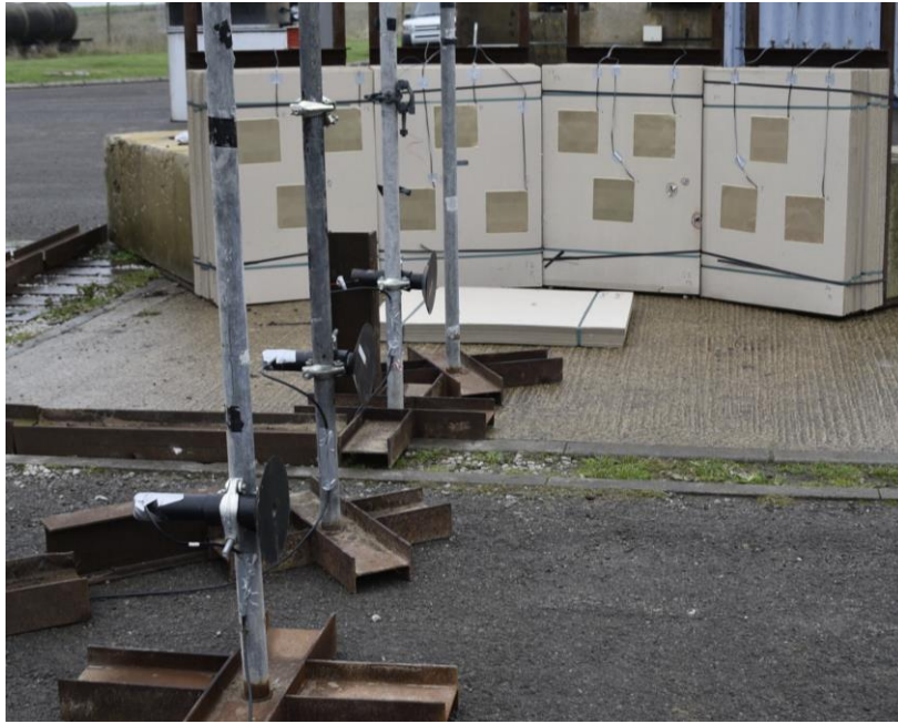
Figure 3 Arena set-up with potentially exposed cable visible
