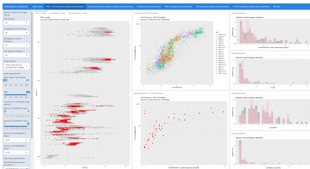
Figure 1: Example dashboard comparing petrophysical, core and petrographic data. Visualisation is built using Flexdashboard library within rmarkdown.(authors own work)
