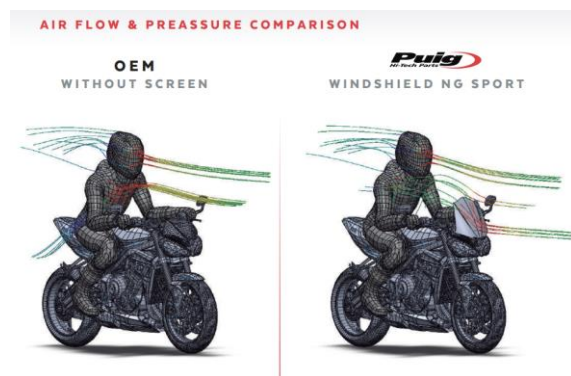
Figure 5 - CFD Flow simulation, screen installed (Puig, 2022)
