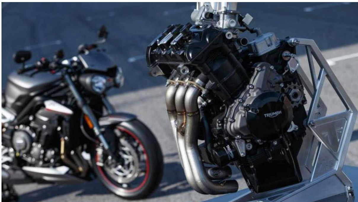
Figure 4 - inline 3-cylinder street triple engine (Staff, 2018)
