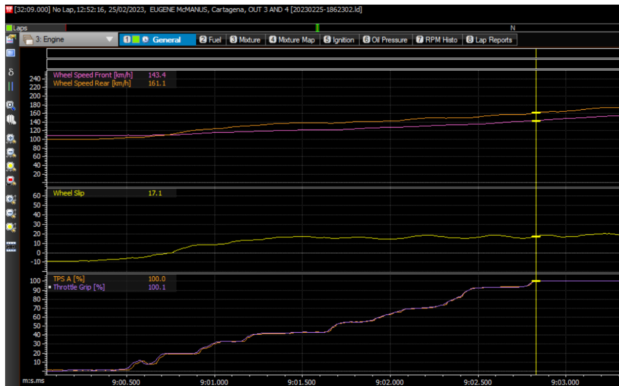
Figure 6 - Wheel Speed F&R, Slip, Tps, Throttle Grip (Harrison, UWTSD, 2023)
