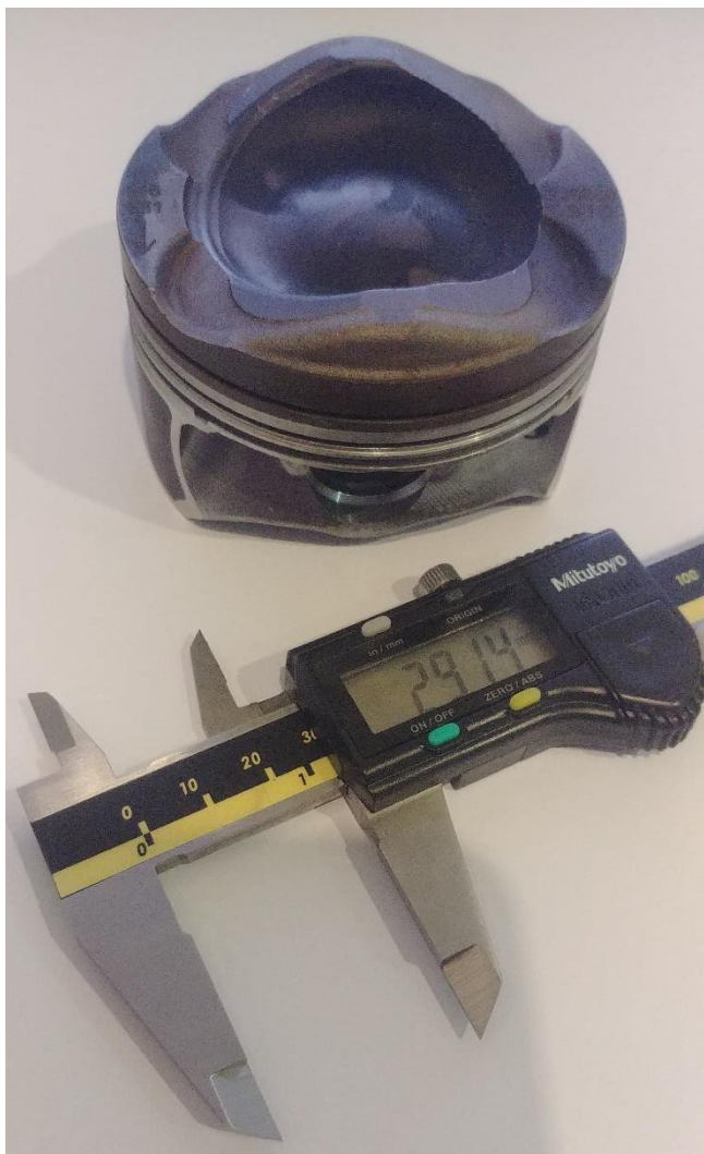
Figure 9: Picture of measuring gauging pin off-set
