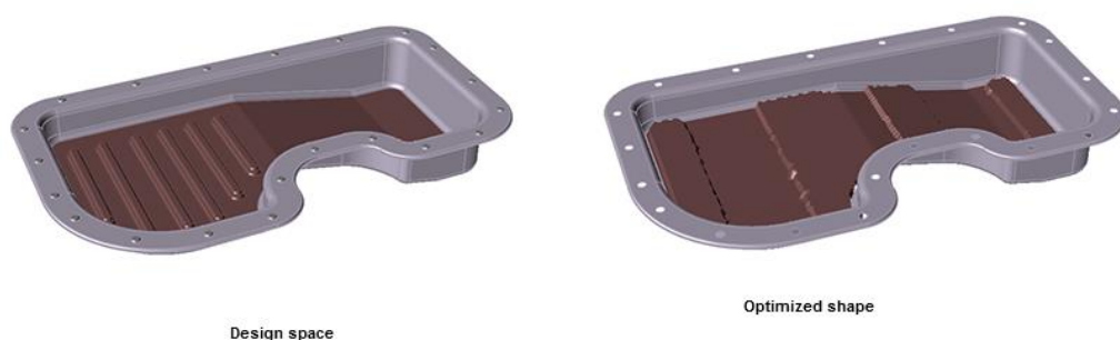
Fig (8) Topography optimisation of sheet metal part. (Structure > Run > Optimization > Topography Optimization, 2020).
