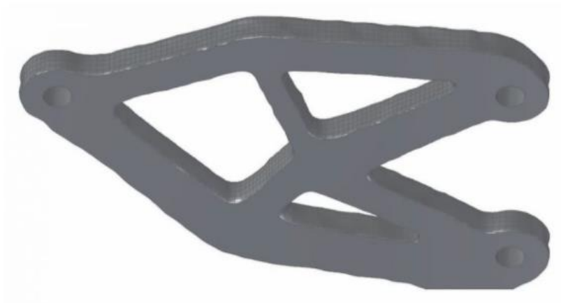
Fig(2) optimised geometry. (Topology Optimisation | Benefits & Disadvantages | Software, 2020)
