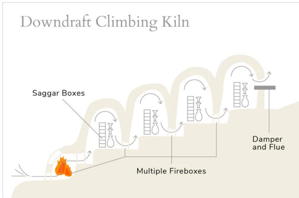
Figure 4: Downdraft Climbing Kiln (Musubi Kiln, 2025)
