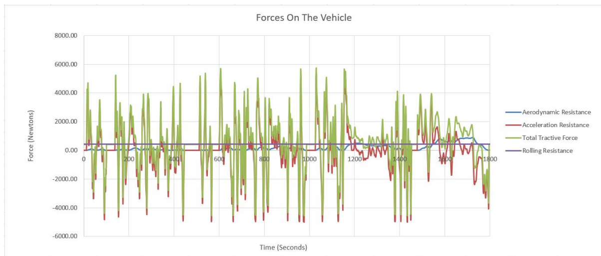
Figure 5, Forces On The Vehicle, Robbie Sandford - WLTC_class_3, 2025
