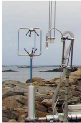
Figure 2: A sonic anemometer used to measure wind speed and direction with no moving parts
