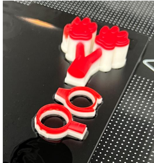
Figure 12 - Support material melting
