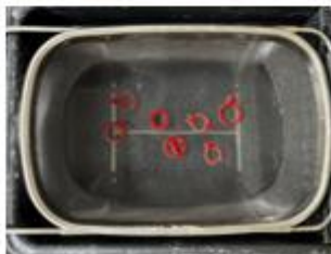
The above image shows a 3D printed wax model in a tray, showing the support material being melted away from the wax.
