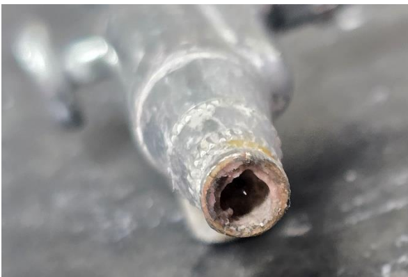
Figure 16 Air compressor nozzle clogged.
