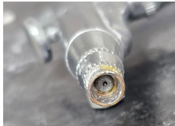
Figure 17 Air compressor nozzle after being cleaned.
